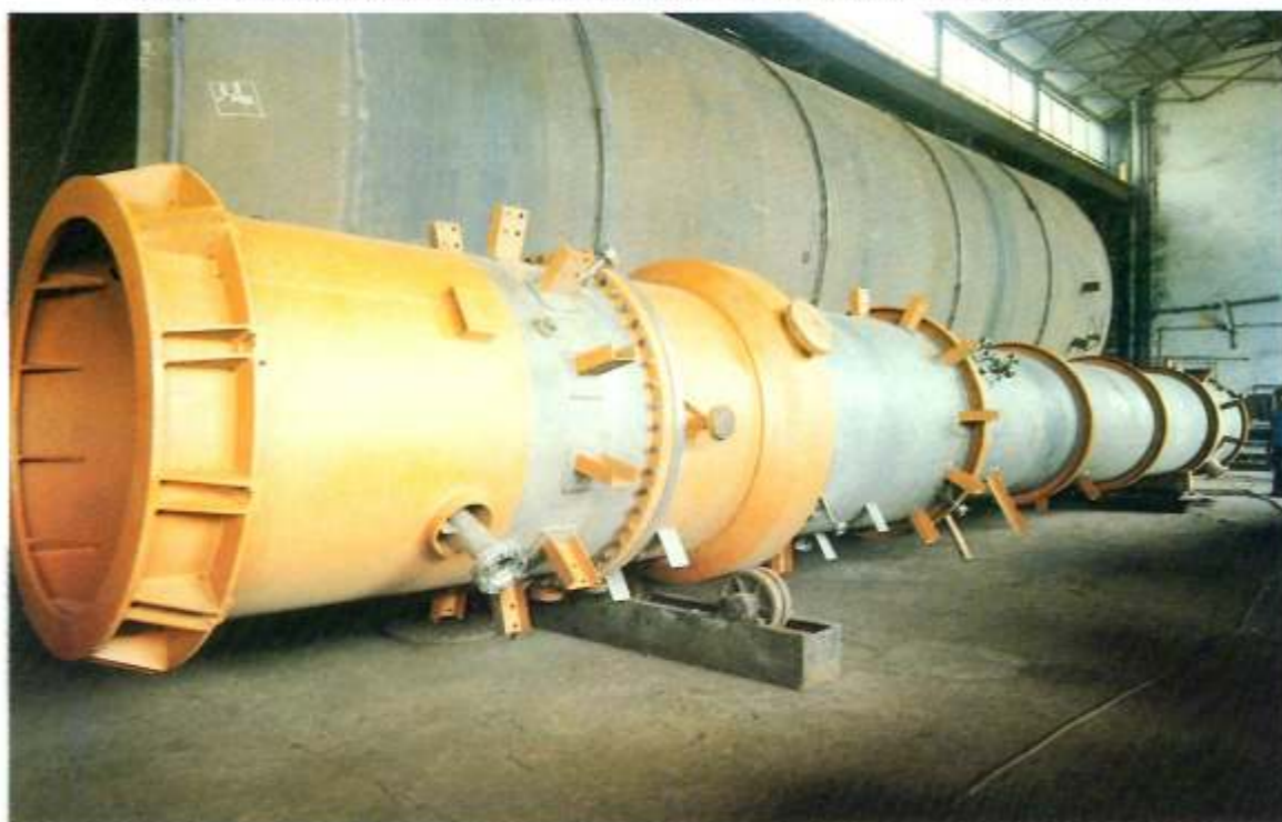
A stainless steel HCN stripper Column designed and manufactured by VTV for National Fertiliser Ltd.'s Bhatinda Plant.
