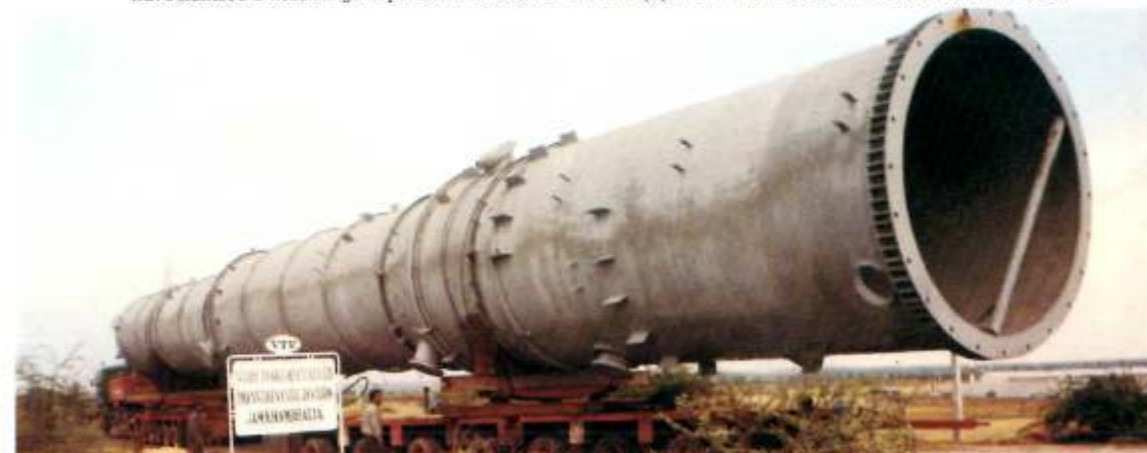
A process column under despatch from VTV's Jamnagar plant for RIL's Jamnagar Petrochemical Complex. VTV's manufacturing facilities have handled a wide range of process columns for the refinery, petrochemical and fertiliser industries since 1963.
