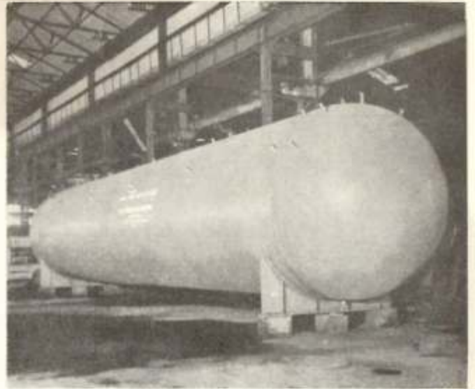
50 tonne LPG Storage Vessel—nine of these were exported to Iraq
